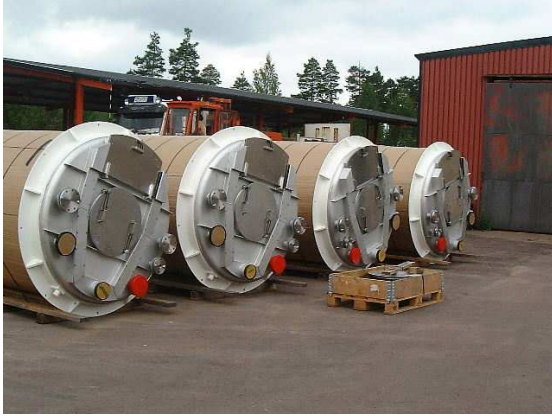
Mixing vessels to be installed in a painting factory in the middle east. 1.4301/304, conical bottom, double shells, large upper flange for a stirrer.
