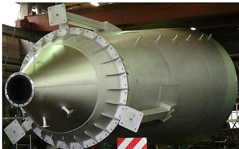
One out of two reactors delivered to a large water work in southern Sweden; largest diameter 4.2 meter, height 10 meter
