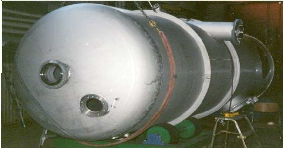
Pressure vessel in 1.4436/316 2.5 % Mo; Separation of filtrate in a paper mill in Tjeckien.
