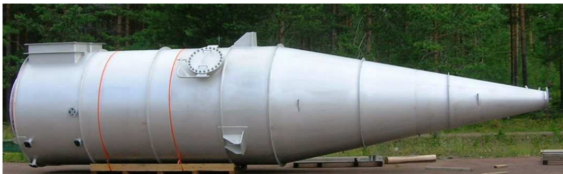
One out of seven stainless process vessels for the manufacture of special products at a paper mill in northern Sweden. Height ca 10 meter, diameter ca 2.5 meter, the conical part is ground and electropolished on the inside. Material: 1.4404/316L.
