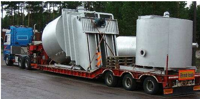
Equipment for water treatment, free standing lamella with flocculation tank, ready for transport to England.
