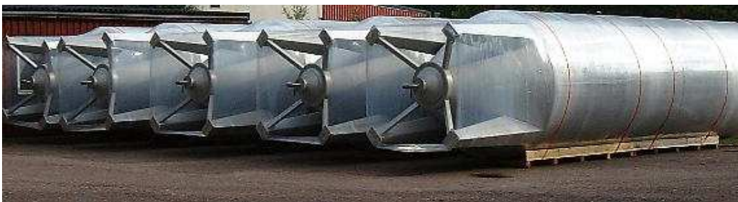
10 meter high stainless steel process vessels for water treatment; Protected by a plastic film during transport. One delivery to China, the other one to England.
