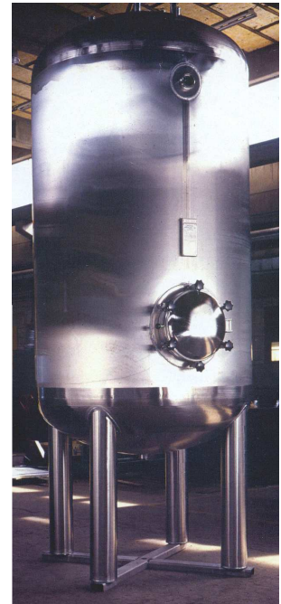
Pressure vessel for ultra pure water for a pharmaceutical plant in Denmark. Inside 1.4436/316 2.5 % Mo, ground to Ra<0.5, Insulated, with the outer shell in 1.4301/304.
