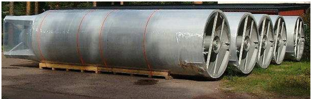
10 meter high stainless steel process vessels for water treatment; Protected by a plastic film during transport. One delivery to China, the other one to England.
