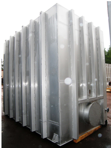
Rectangular tank, with supports on the outside, for installation in a painting factory in central Sweden.
